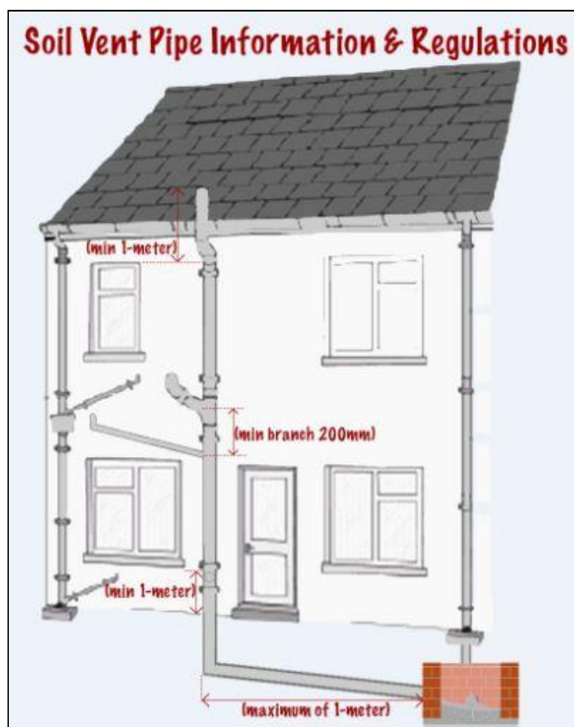
12.0 Item 1(Picture) Soil pipe system
