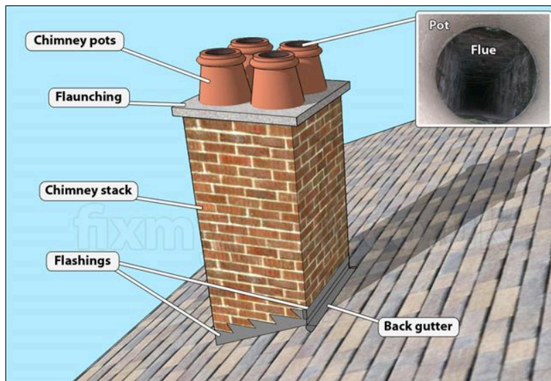
9.0 Item 1(Picture) Chimney components
